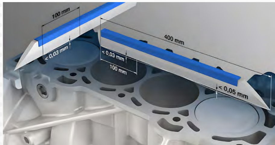
PRO TIP: Maximum values for component unevenness and distortion for passenger cars. Practical measurement using a straightedge and the light-gap method.
