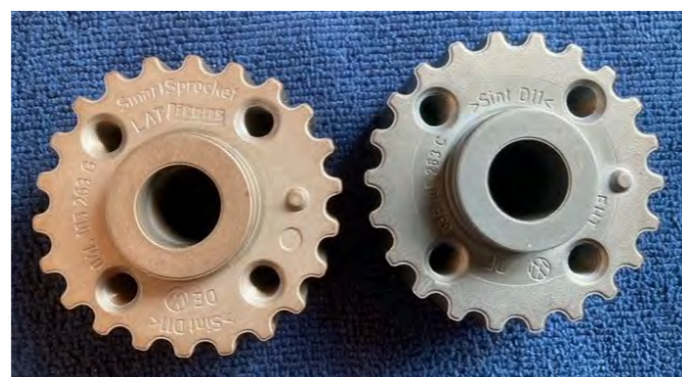
Oval / 'Smart' camshaft sprocket vs traditional round sprocket
